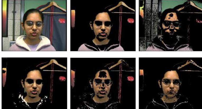
**Fig. 6.** Results from the VALID database with a complex background. From left to right, top to bottom: original image; results for explicit RGB rules; results for SPM in RGB,  $T = 0.15$ ; results for SPM in HSV,  $T = 0.05$ ; results for SPM in YCbCr,  $T = 0.03$ ; results for our model.
